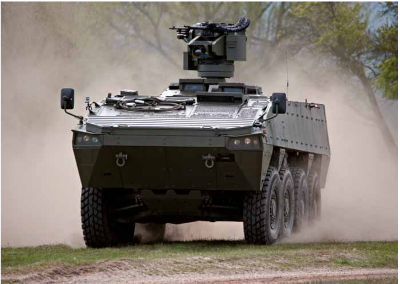
Trackfire RWS SILOS with GMG and MAG58 on Patria AMV
