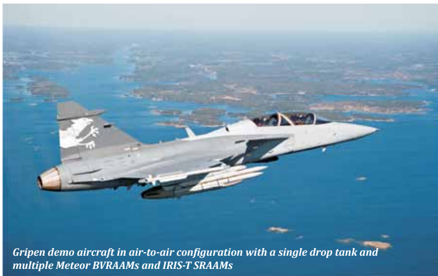
Gripen NG demo aircraft pictured with ‘swing role’ payload – LGBs, Meteor BVRAAMs, IRIS-T SRAAMs and underwing drop tanks.
