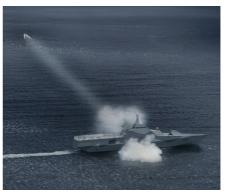
Visby-class corvette's all-composite carbonfibre hull and superstructure is not only lighter than steel, but also comparable for fire resistance and ballistic properties, and superior to steel for vulnerability to blast and underwater explosions. In terms of life cycle costs, the carbon-fibre composite is entirely superior to steel and aluminium for fatigue. And the superior corrosion resistance reduces the platform lifecycle costs even further.
