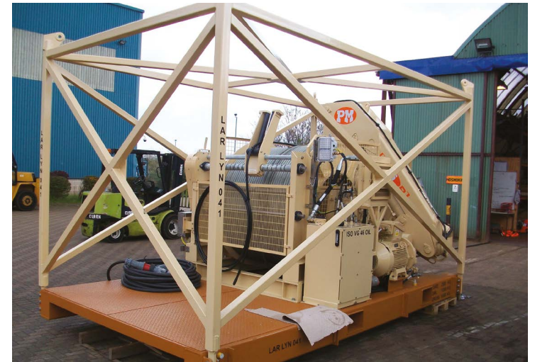
Hiab crane LARS stowed for transport
