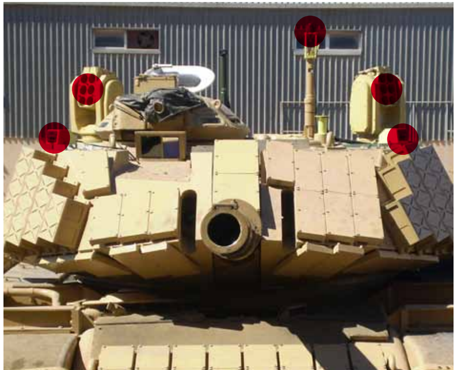
LEDS-100 with high speed directed launchers integrated on MBT.
