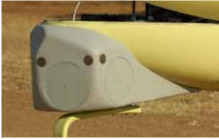
Antenna Array with low band (0.5-6 GHz) and high band (6-18 GHz) antennas.
