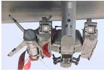
*BOL integrated in LAU-128 launcher on F-15.*
