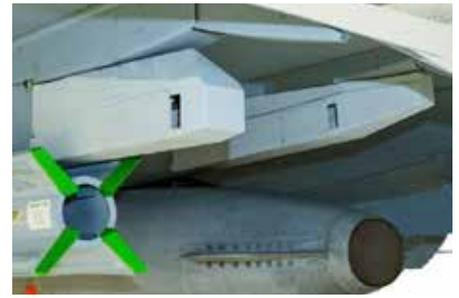
*Installation of mock-ups for new internal BOL dispensers.*
