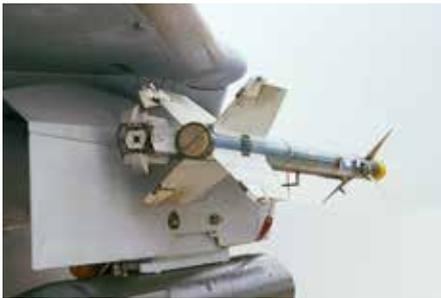
*BOL integrated in LAU-7 launcher on F-14 as it was installed.*
