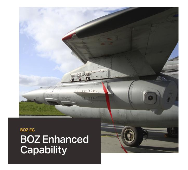
**BOZ EC** is a highly effective, combat proven, countermeasures pod for high performance aircraft. BOZ EC has extended pre-emptive and reactive self-protection capabilities through missile warning and flare cocktail dispensing.
