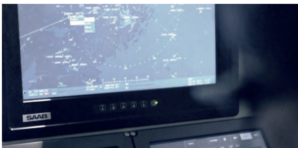
Sirius enables coordinated mission planning and execution, utilising available sensor resources connected through a network. Sensors can be remotely controlled and sensor data is processed and consolidated into a common situational picture, including platform classification and geolocation, used for tactical objectives and reported to an external C4I system.
