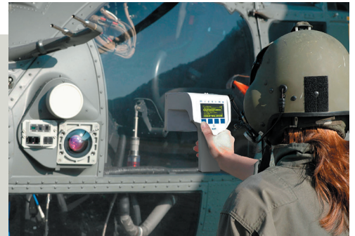
Missim, one tester for all sensors (from RUAG)
