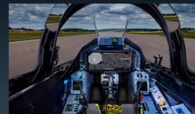
**AEL SISTEMAS:** *Wide Area Display, Head-up Display e Helmet-Mounted Display.*
