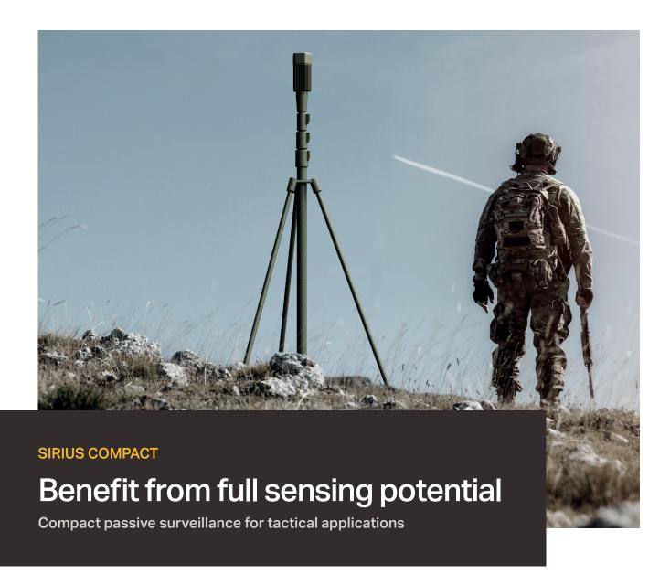
**Sirius Compact** is a modular and scalable passive Electronic Warfare (EW) sensor network which provides a true force-multiplier by enhancing situational awareness through detection, tracking and classification of radar and datalink emissions.
