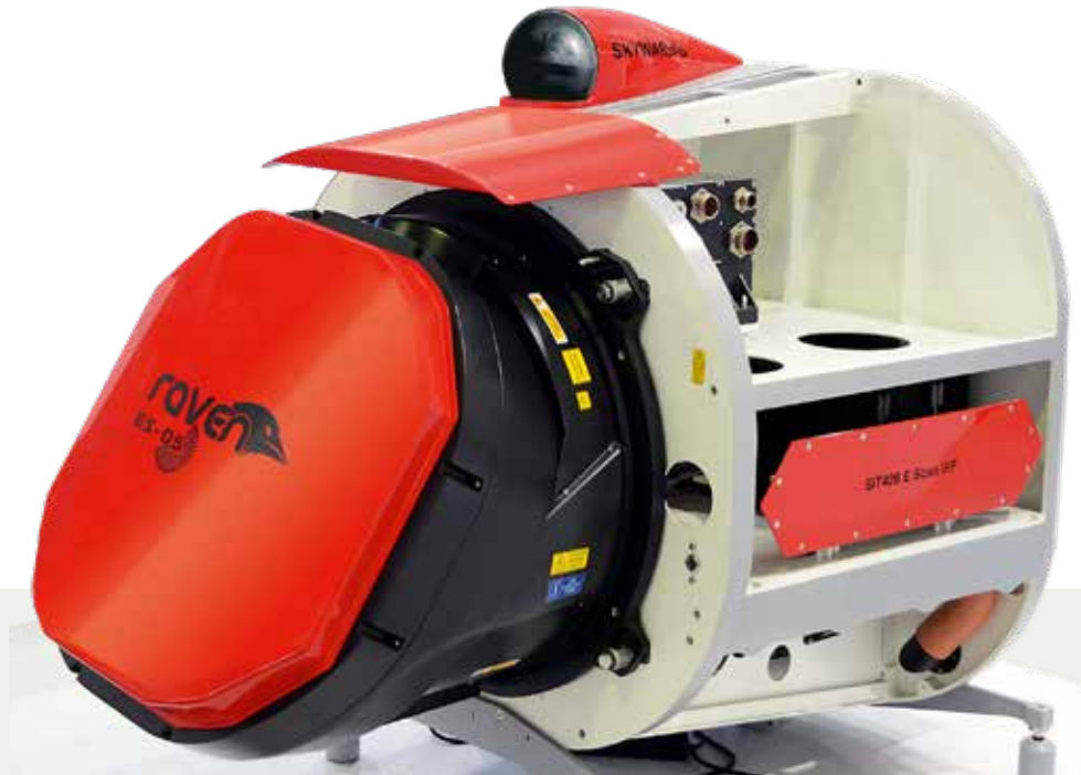
The Active Electronic Scanned Array Raven ES-05, Infrared Search and Track (IRST) Skyward-G and the IFF SIT426 E Scan antennas.
